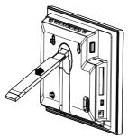
**5** Slide the power switch to the **ON** position. The frame automatically turns on and starts playing a slideshow of the pictures stored in internal memory. This slideshow is called Demo mode.
